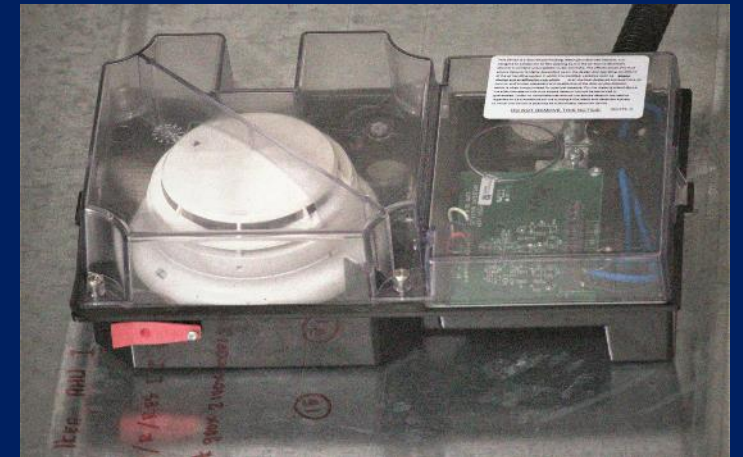
Smoke Duct Alarm
